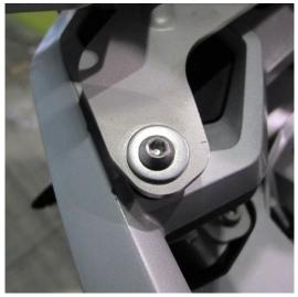
9. Set the rear screws (M6x65) with the special washers and thighten carefully but **not completely**.
