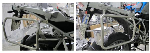
8. Mount the traverse and tighten all bolts firmly.
