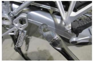
6. Place the U-Form washer to the front bolt tighten the bolts slightly.
