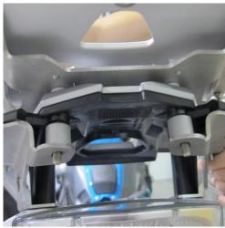
12. Set the washers and nuts (M6) for all front and rear bolts and thighteen firmly.
