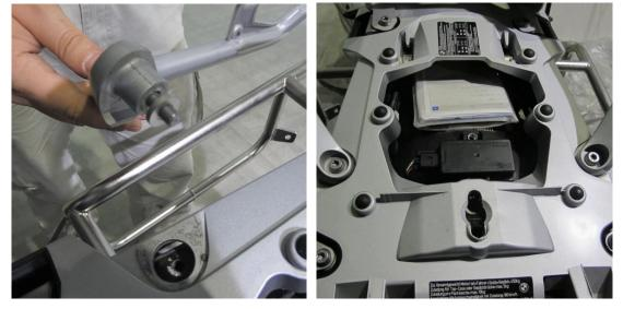
6. Check the correct position of the handle bar with the black plastic support.
