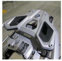
8. Set the front screws and washers and thighten slightly. (M6x50)
