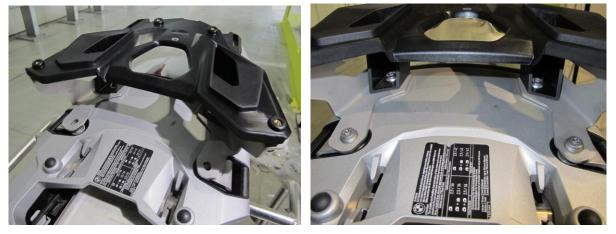
5. Place the other 2 thin alu. washers (3mm.) as shown in the picture and place the rear passenger handlebar carefully to the bike. Left and right screws simultaneously. Pay attention that the washers do not fall inside the rear section of the bike. If so, you can pick them up after you remove easly the big grey cover.
