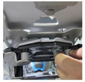
11. Now screw the rear bolts completely and thighteen firmly.
