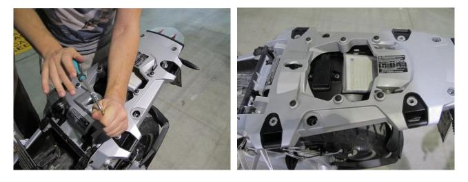
2. Open the package with all the hardware inside and seperate the 4 joint parts with numbers on back sides.
