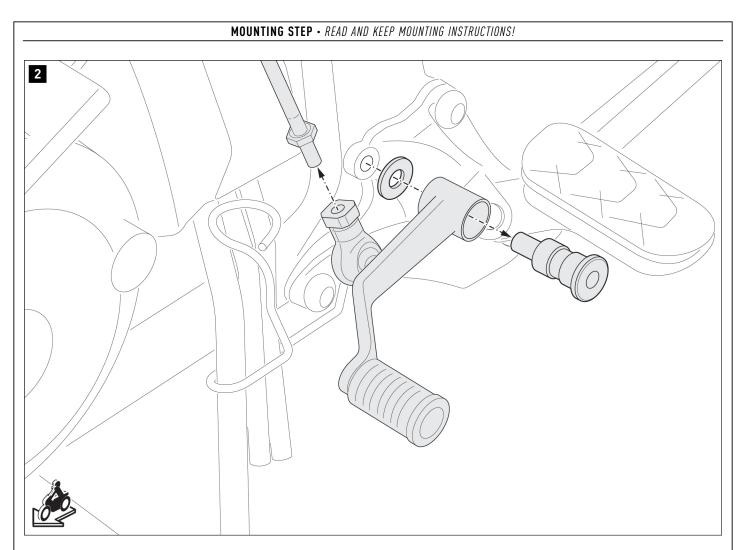
Loosen the parts shown; remove the original gear lever from the vehicle.
