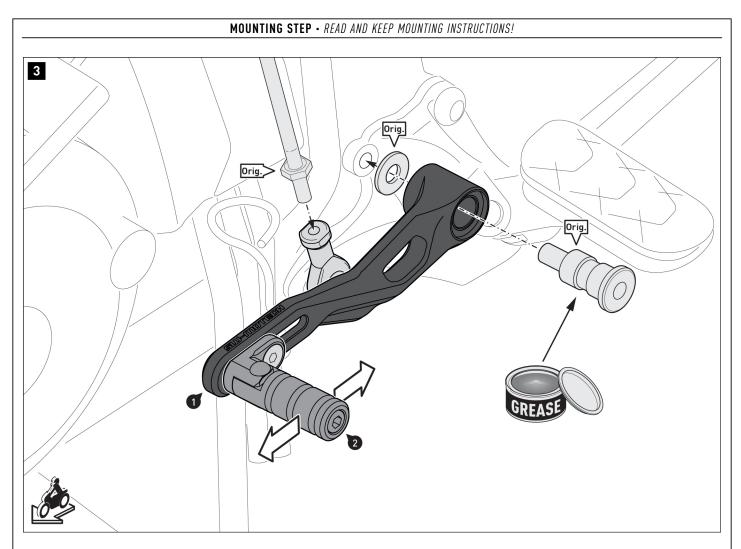
Screw the original deflection rod (Orig.) to the gear lever (1) (min. 6 thread); secure using the corresponding nut.
