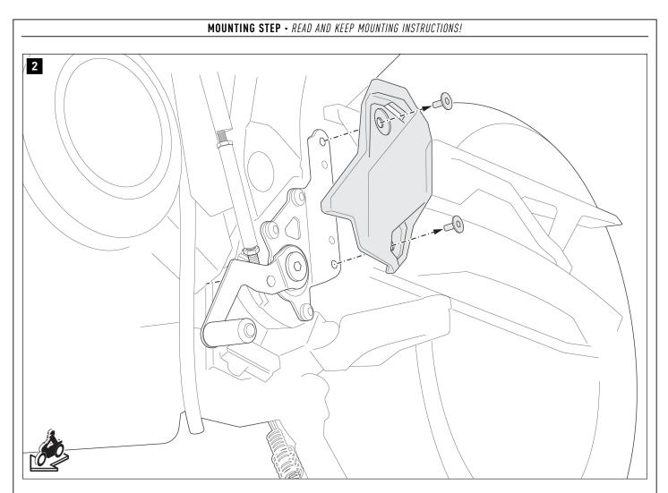
Loosen the screws shown and remove the heel guard from the vehicle.
