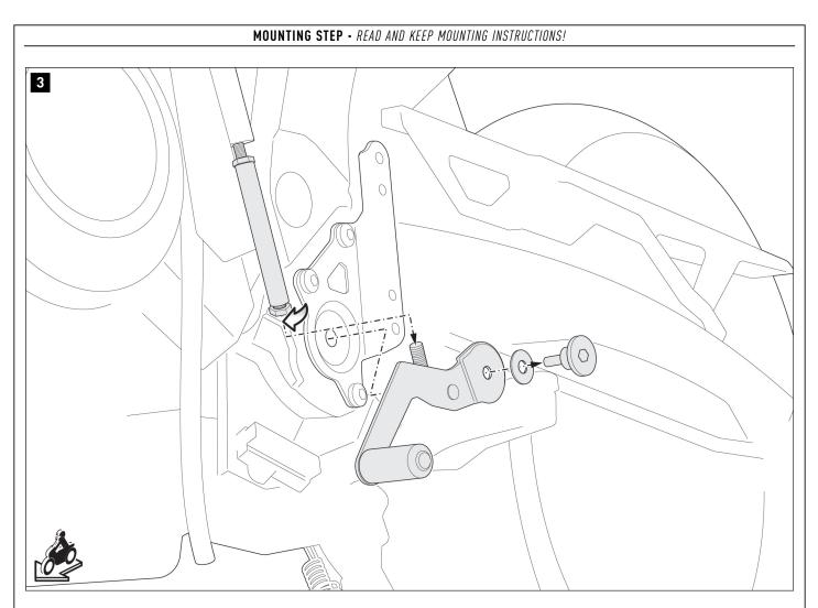
Loosen the screw and nut shown and remove the original brake lever from the vehicle.
