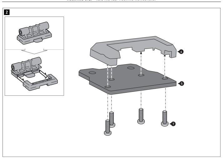
▲ NOTE: Holding frame (6) and slide-in frame (2) are delivered assembled!
