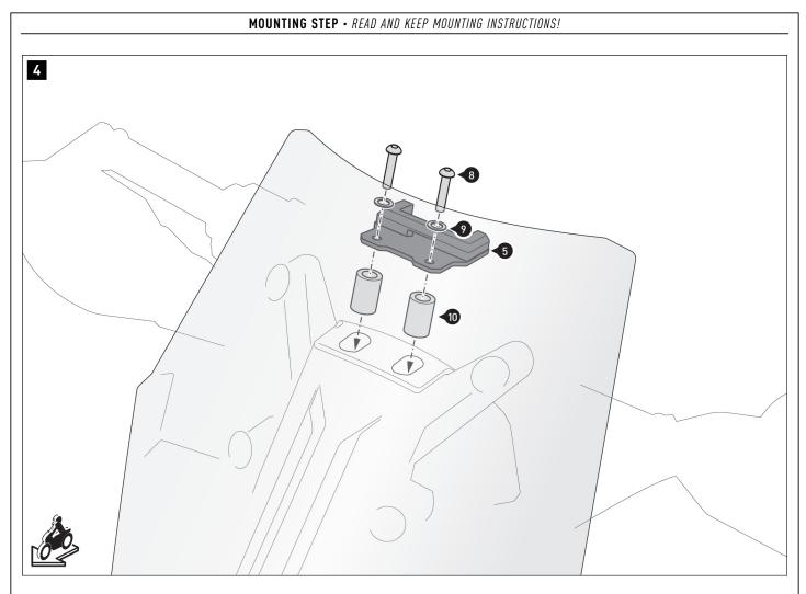
Screw the mounting bracket (5) to the vehicle. **A** WARNING: Use a liquid threadlocker! Tighten the screws (8) according to the manufacturer's instructions.
