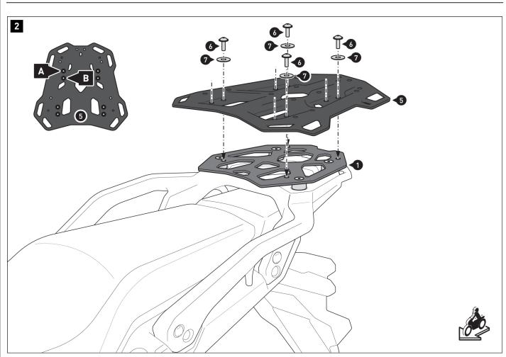
$\triangle$  **NOTE:** Depending on the space available, screw the rack to **mounting position** (A) or (B), as indicated in the detailed drawing.
