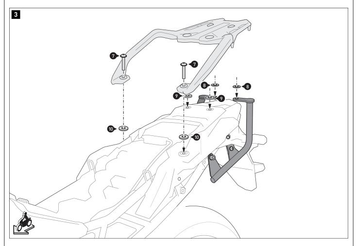
$\triangle$  **NOTE:** When connecting to the SW-MOTECH side carrier, spacers (9) and (10) are no longer required. In their place, mount the side carrier using the parts from the rack.
