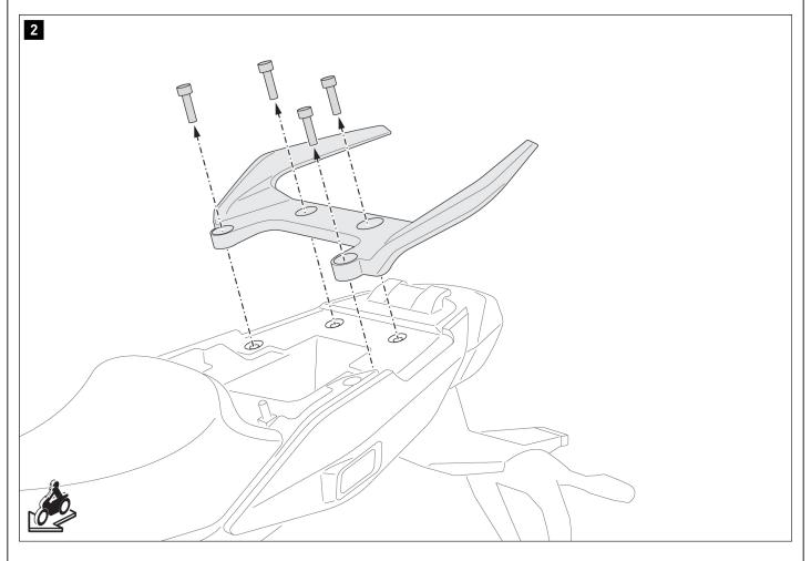
Loosen the screws from the attachment points indicated and remove the passenger grip from the vehicle.
