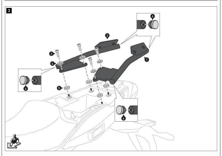
Insert the plastic plugs (6) into the ends of mounting struts (1) and (2).
