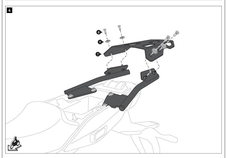
Screw the rack (7) onto mounting struts (1) and (2). **A WARNING:** Use a liquid threadlocker!
