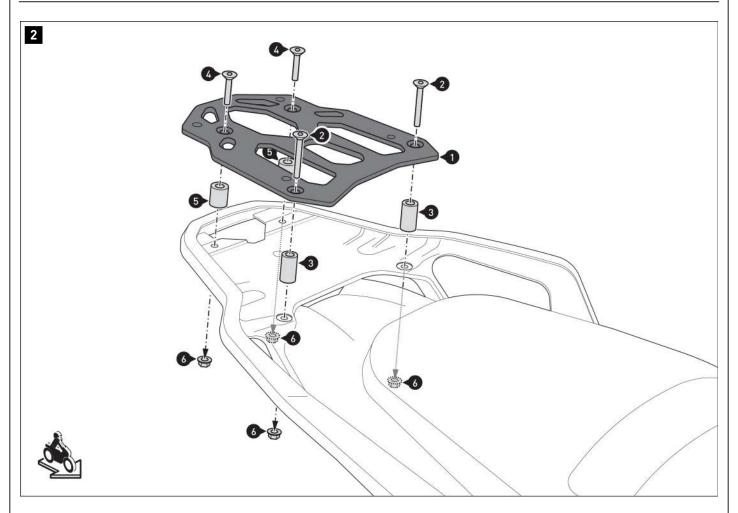
Mount the mounting bracket [1] on the rack. Tighten the screws [2] and [4] as specified in the mounting instructions.
