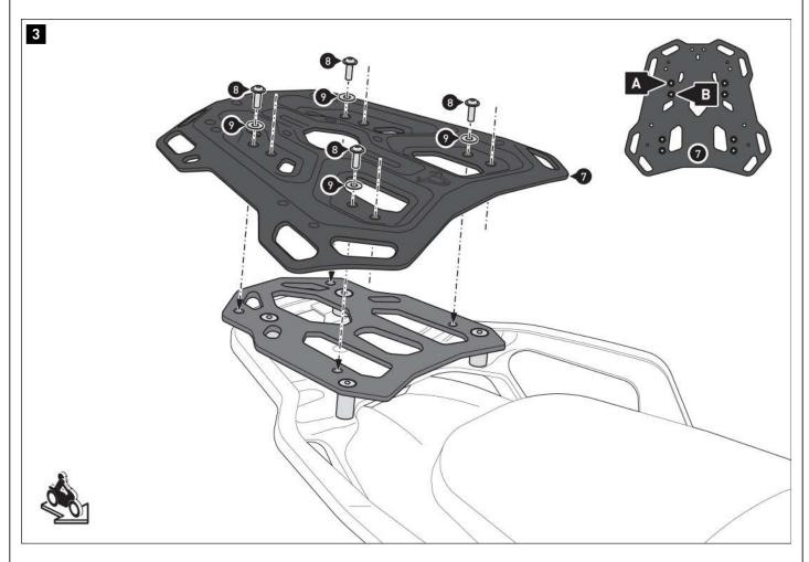
$\triangle$  **NOTE:** Depending on the space available, screw the luggage carrier (7) to the marked mounting position **(A)** or **(B)** as shown in the detailed drawing.
