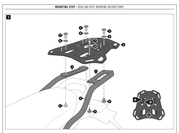
▲ **NOTE:** Depending on the space available, bolt the rack to mounting position (A) or (B), as indicated in the detailed drawing.
