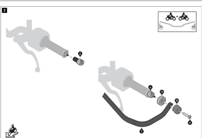
Remove the original end weights and handguards if mounted. Make sure the handlebar ends and the inside of the handlebars are clear.
