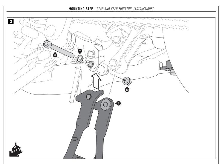
Screw the centerstand (1) to the vehicle. Tighten the screw (8) as specified in the mounting instructions.
