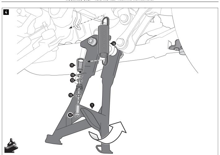
Fold up the centerstand (1) and hold it in position using a suitable jack.
