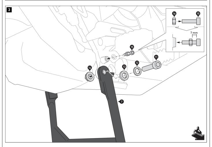
Screw the centerstand (7) onto the right-hand side of the vehicle. Now tighten the screws (8) and (11) according to the manufacturer's
