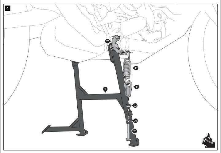
Hang the spring link plate (17) on the screw (15).
