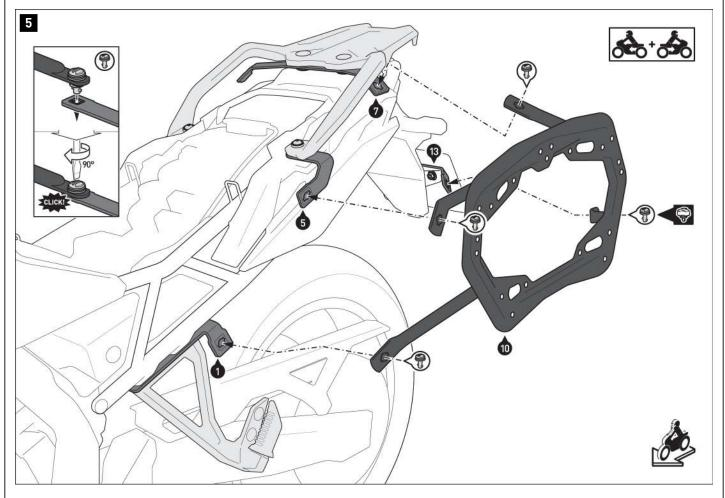
$\triangle$  **NOTE:** The SW-MOTECH anti-theft protection devices are available separately; mount the anti-theft protection devices on both sides at the indicated position. a
