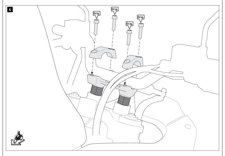
Screw the handlebars back to the vehicle according to the manufacturer's instructions.
