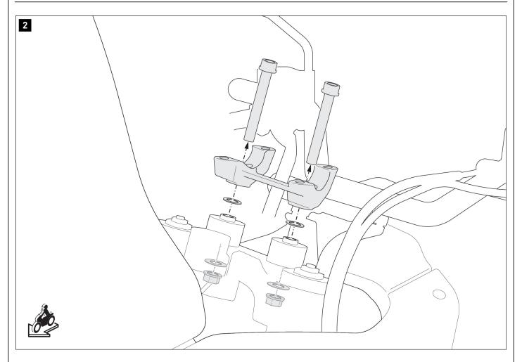
Unscrew the two screws shown and remove the handlebar bridge from the vehicle.
