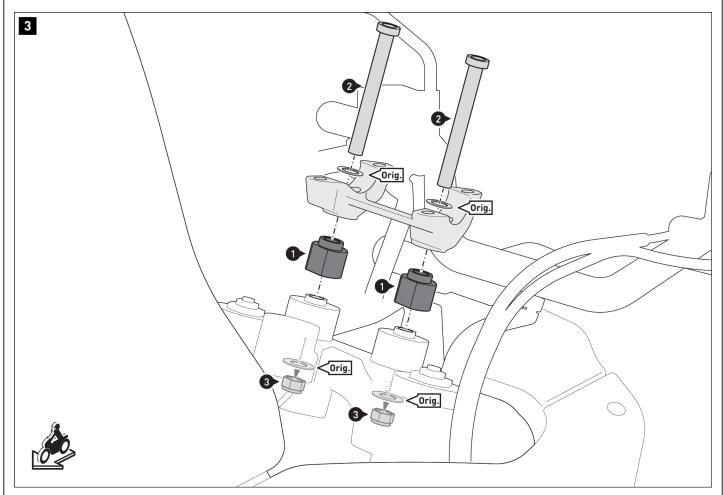
Screw the bar risers (1) to the vehicle using the original washers (orig.). Tighten the screws (2) according to the manufacturer's instructions.
