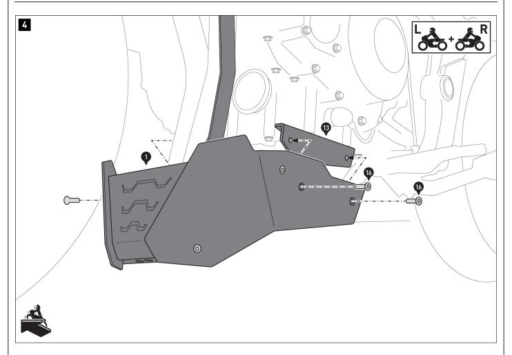
Use the screws (16) to attach the engine guard (1) to the mounting brackets (12) and (13) on both sides.
