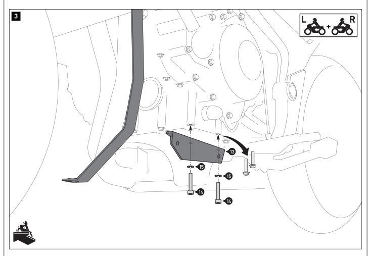
Remove the screws from the attachment points indicated on both sides of the  $% \left\{ 1,2,...,n\right\}$
