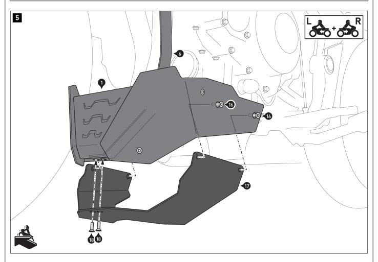
Screw mounting bracket (17) to mounting bracket (6) and to the inside of the engine guard (1). **A WARNING:** Use a liquid threadlocker!
