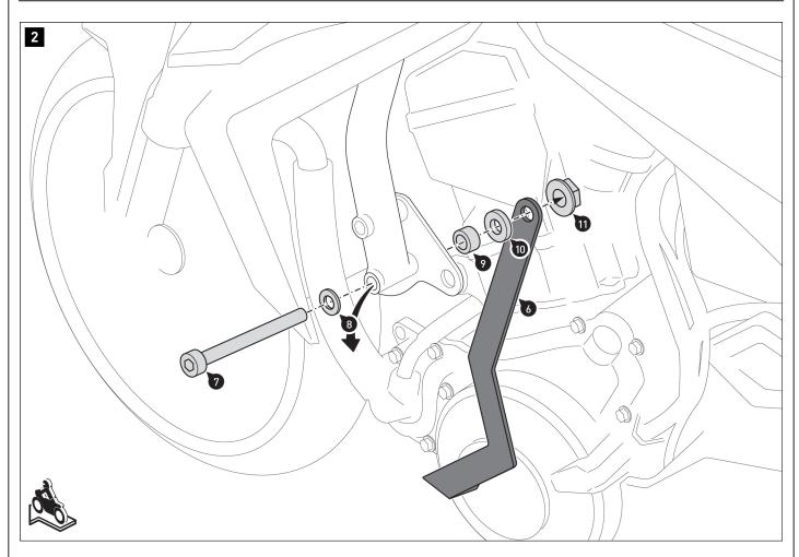
$\triangle$  **NOTE**: If installed at the same time as the SW-MOTECH crash bar, the spacer (10) is not required. Instead of the spacer, use the piece from the crash bar.
