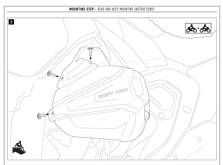
Undo the screws indicated on **both sides** of the cylinder panelling.
