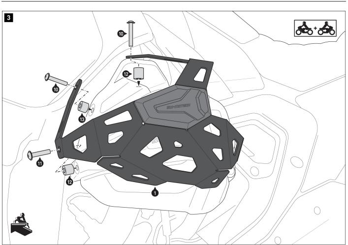
Screw the mounting bracket (1) to the **left** cylinder and the mounting bracket (2) to the**right** cylinder. A **NOTE:** Note the asynchronous installation of the mounting brackets (1) and (2): Use the screw (14) and spacer (15) on the **right** side of the vehicle at the **front** attachment point and the spacer (13) at the **upper** attachment points. A **WARNING:** Use a liquid threadlocker! Tighten the screws (10), (11), and (14) according to the manufacturer's instructions.
