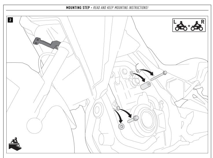
$\pmb{\mathbb{A}}$  WARNING: Do not start fitting the right-hand crash bar until you have finished fitting the left crash bar!
