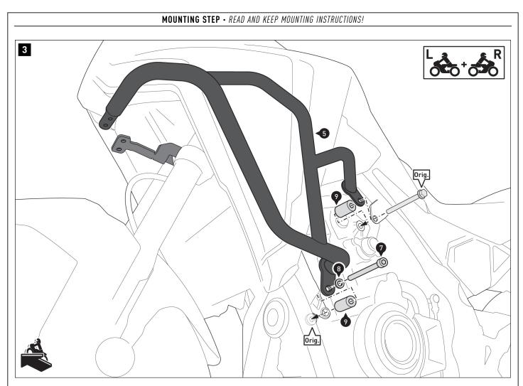
Screw the crash bar halves (5) and (6) with the original parts shown (Orig.) screws. **A** WARNING: Use a liquid threadlocker! In this step, hand tighten the screws until both crash bars are aligned.
