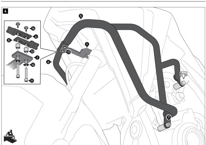
Screw the crash bar halves (5) and (6) to the mounting bracket (1).
