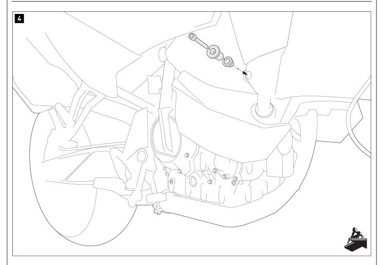
On the right side of the vehicle, remove the screw from the attachment point shown.
