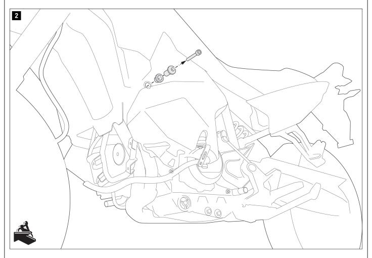
Remove the screw shown on the left side of the vehicle.
