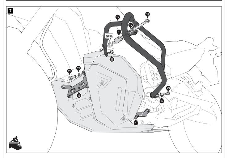
Screw the left half of the crash bar [17] to the mounting bracket [1], to the cross connector [13], and to the original damper (Orig.) on the vehicle.
