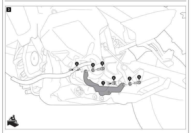
Screw the mounting bracket [1] onto the left side of the vehicle. **A WARNING:** Use a liquid threadlocker!
