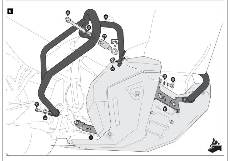
Screw the right crash bar half (24) to the mounting bracket (7), to the crossbar (13), and to the original damper (Orig.) on the vehicle.
