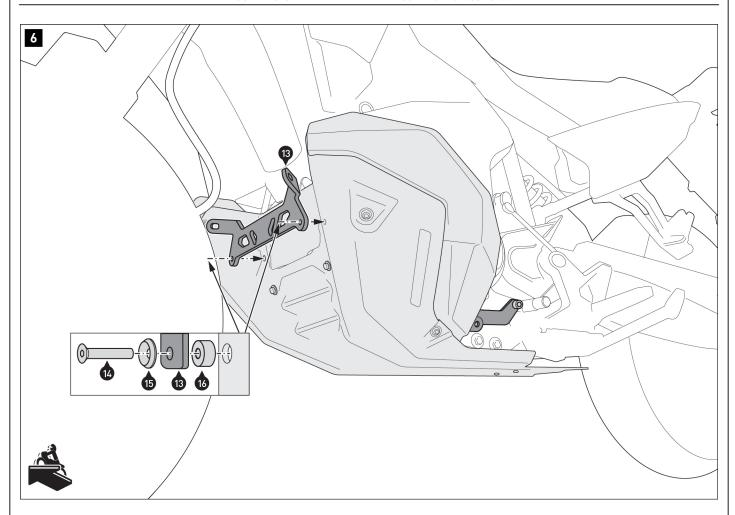
Reattach the original engine guard to the vehicle. **A** WARNING: Use a liquid threadlocker!
