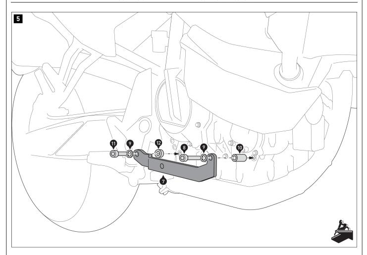
Screw the mounting bracket [7] onto the right side of the vehicle. **A WARNING:** Use a liquid threadlocker! Do not tighten the screws yet.
