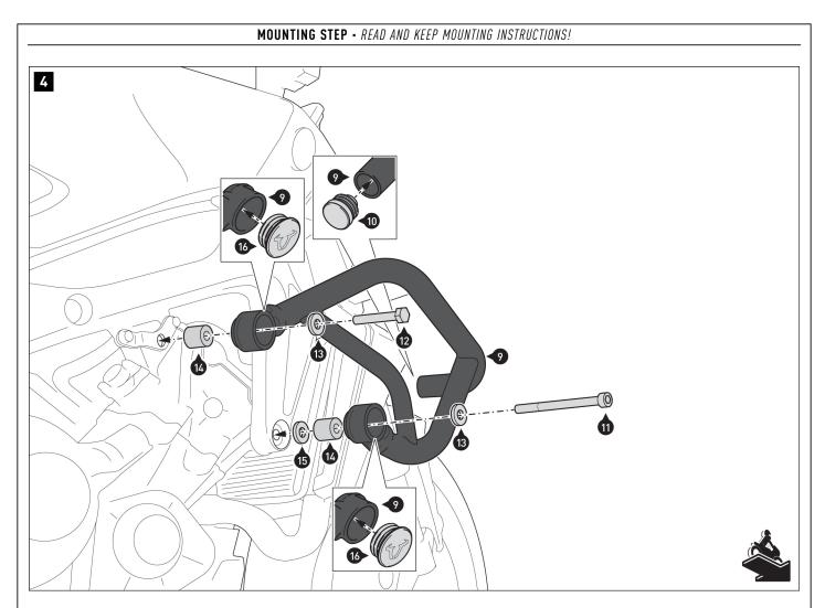
Insert the plastic plugs (10) into the opening of the crash bar (9).
