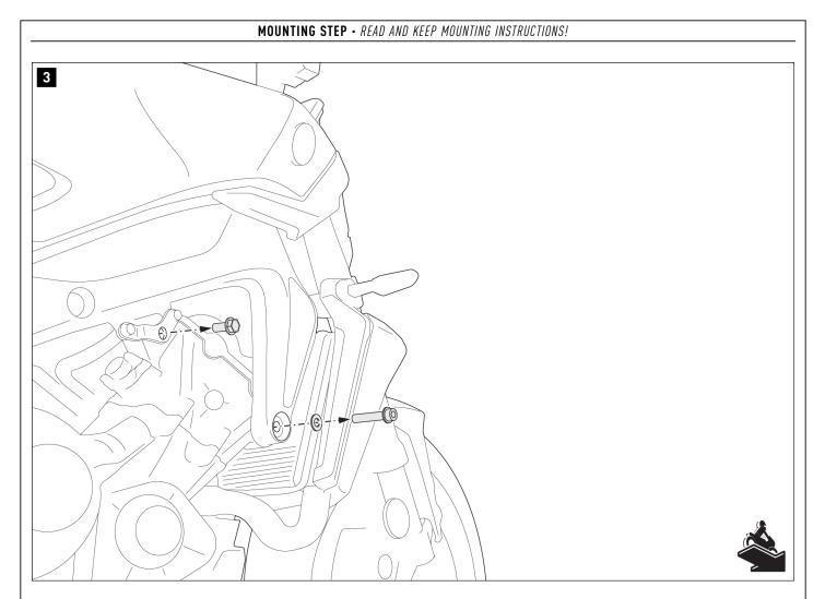
Remove the screws from the mounting points shown.
