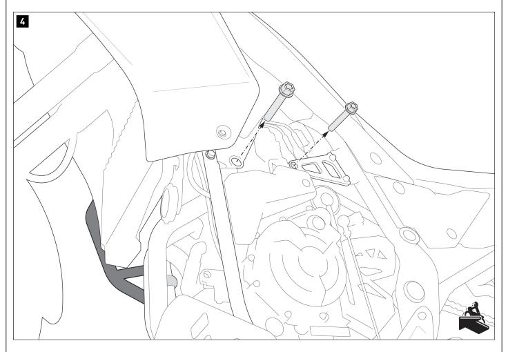
Remove the two screws indicated on the left side of the vehicle.
