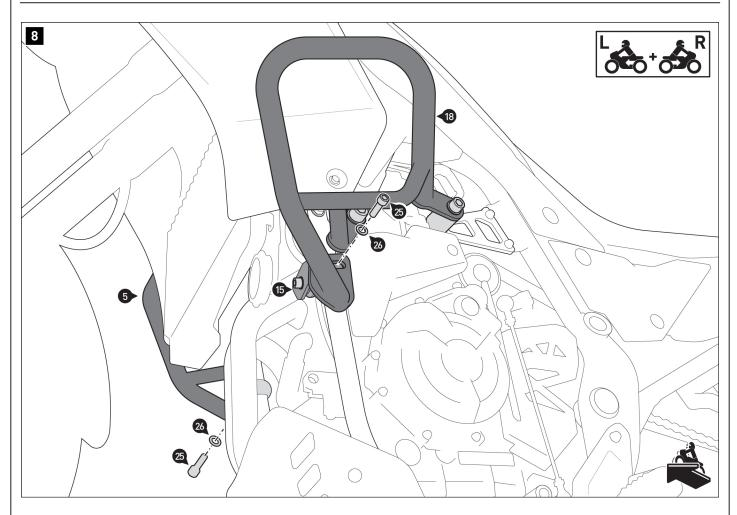
Screw the crash bars (5) and (18) to the mounting brackets (15). **A WARNING:** Use a liquid threadlocker!
