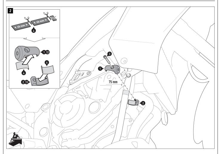
Cut each of the rubber strips (4) into two 40 mm pieces (the rest is no longer
