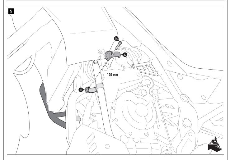
Screw the clamps (12) and (13) to the vehicle frame.
